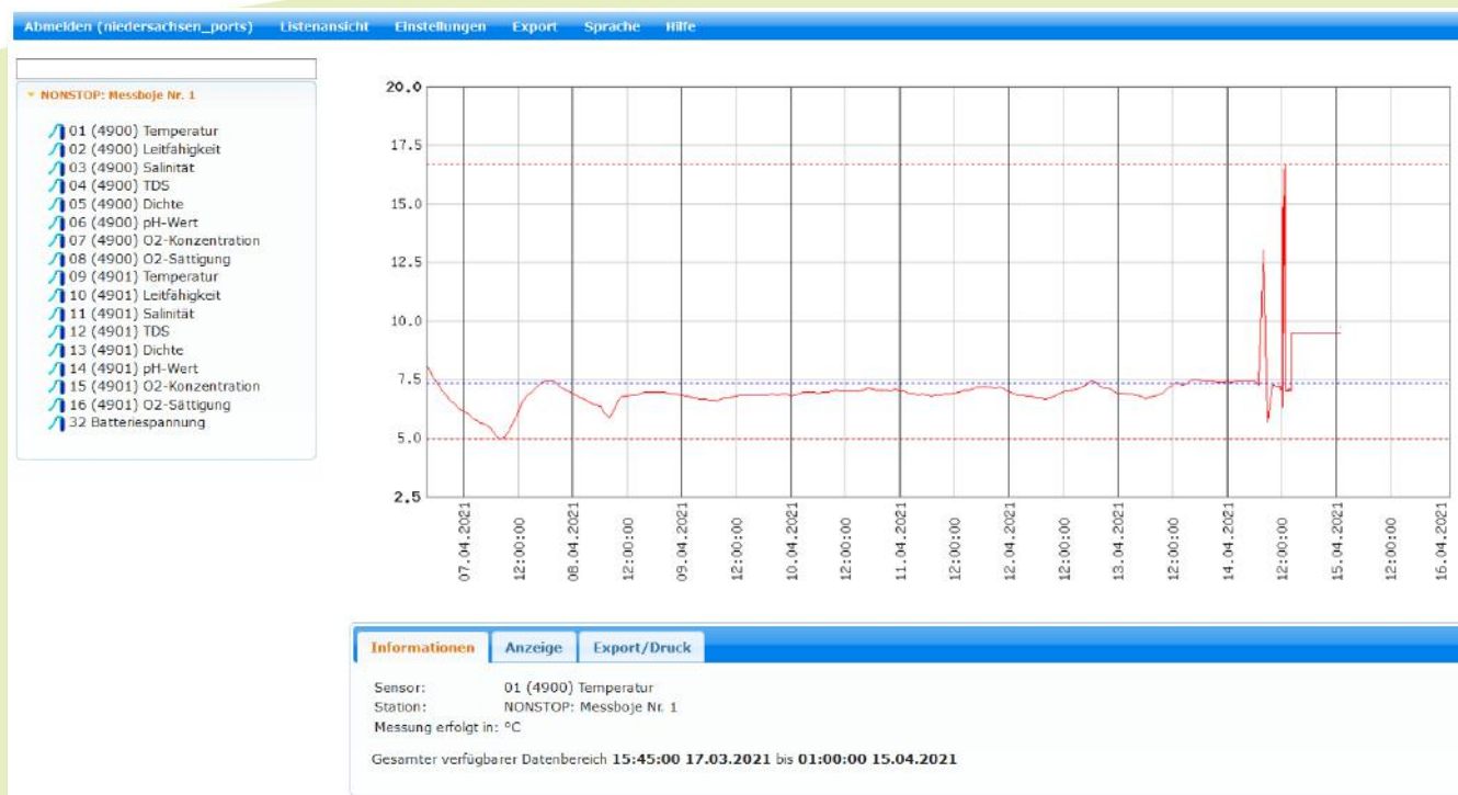
Figure 37. Representation of temperature measurement from the measuring buoy in the SEBA Hydrocenter software.
