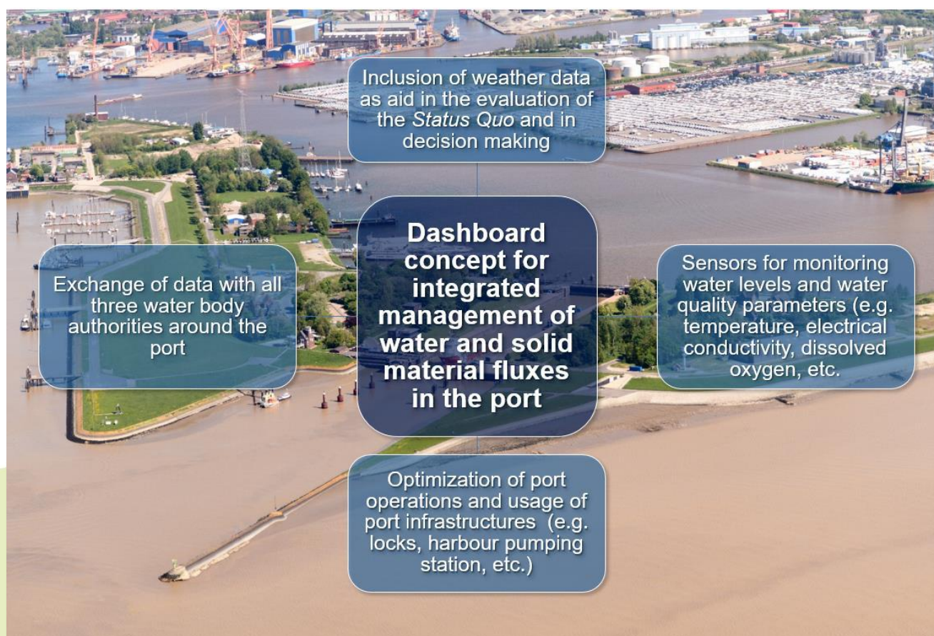
Figure 8. Schematic representation for the concept of a dashboard system for the Port of Emden.
