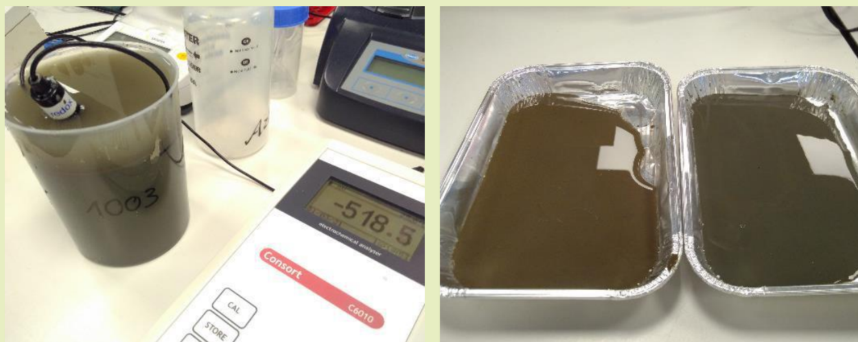
Figure 17. Examples of direct measurements of fluid mud properties. Left: Redox potential of sample from IH location. Right: Visual observation of fluid mud samples. Brownish discoloration is typical for more oxidized fluid mud from GS and grey colours indicate more reduced oxygen in fluid mud from IH. Credits: TU Delft.
