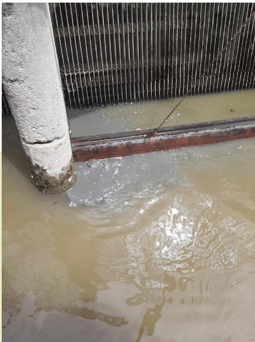
Figure 10. Panel board used as a sediment barrier in the inlet area of Pump 1 at the port's pumping station for the field test.
